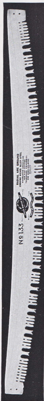
No. 133. Perforated Lance Tooth Saw. Four Cutting Teeth to each Raker.
